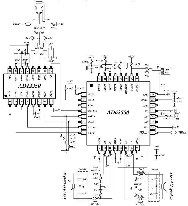
Note6: These capacitors should be placed close to speaker jack as possible, and their values should be determined according to EMI test results.
