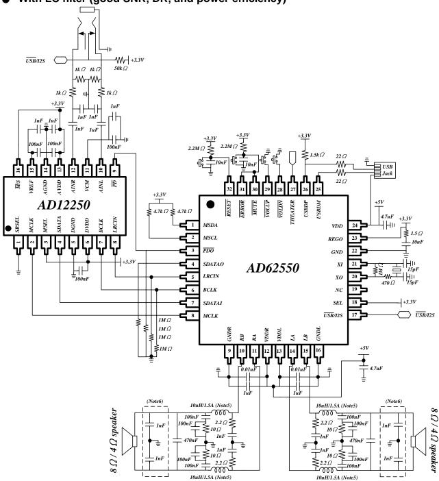
Note5: When  $8\Omega$ 's loads are used, the 22uH/0.8A inductors are suggested.
